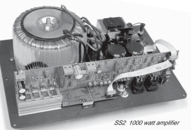
Since switching amplifiers are very high efficiency, about 92% in this case, very high power and currents can be delivered without large heat sinks, fans or additional power supply capacity for large amounts of waste heat. This type of amplifier is ideal for subwoofer applications since the amplifier does not have to deliver significant power at high frequencies.
